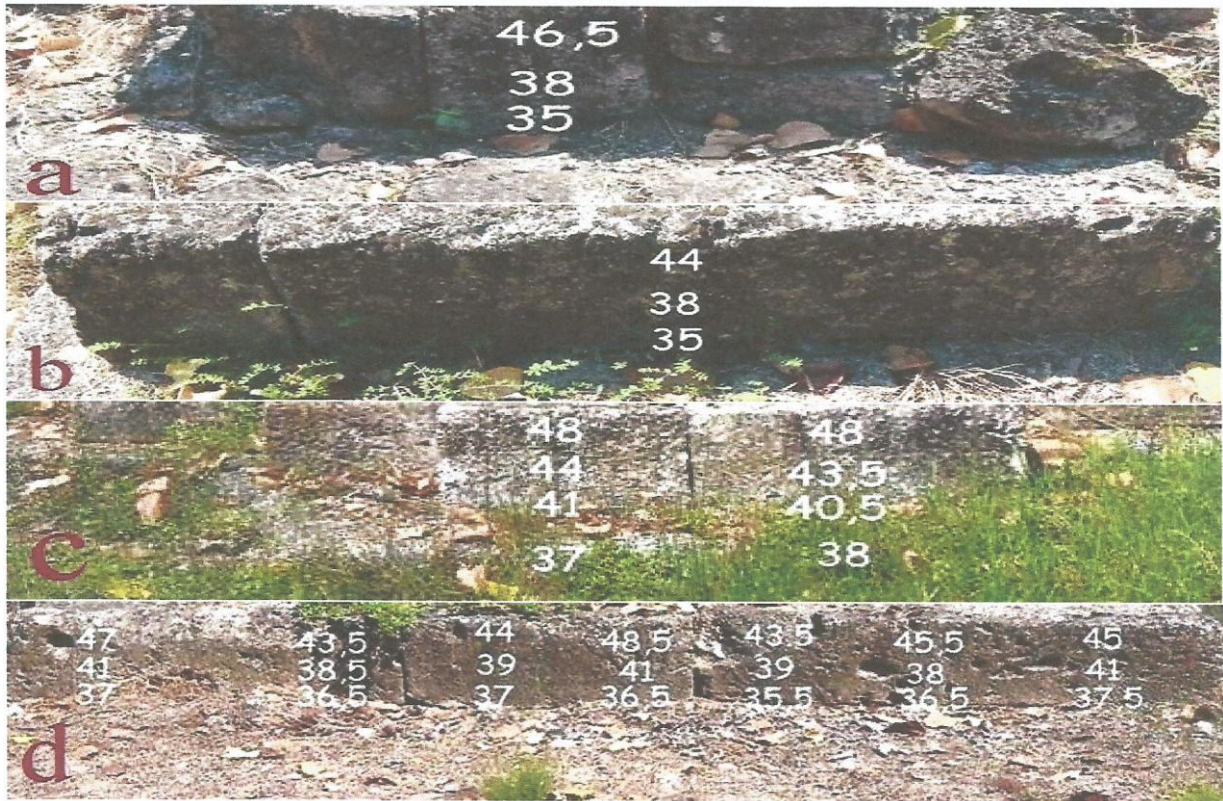
Figure 7 IR thermometer measurements, sunny conditions, Demeter sanctuary, Altar, a) north side, b) east side, c) south side, d) west side.
